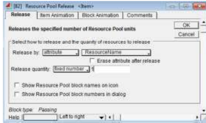
Figure 4-17: “Resource Pool Release” block that releases resources after a finishing process.
