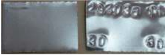
Figure 3-5: Aluminium tag sheet before and after engraving numbers.
