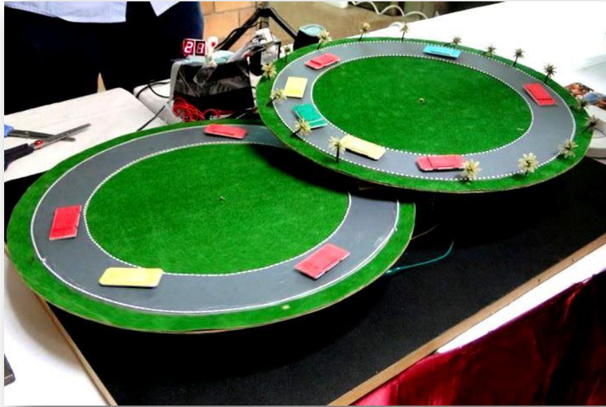
Figure 10-8: The prototype representing FPGA control in a pre-timed traffic control system
